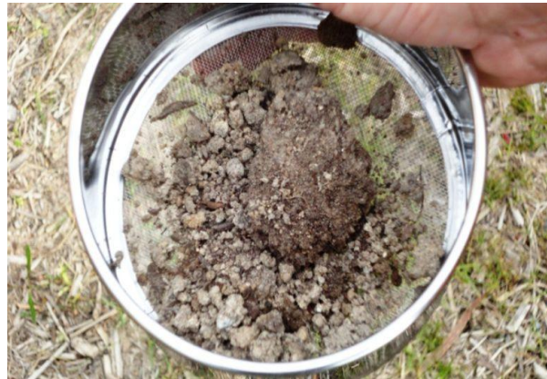
Figure 1. Soil sampling is a basic technique of mineral exploration. Cheaper than drilling, sampling can be used to quickly establish the existence and extent of hoped for mineralisation. Image reproduced from 'Geology for investors' ( https://www.geologyforinvestors.com/rock-and-soil-sampling-the-key-to-most-exploration-projects/ ).
