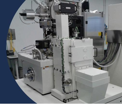
Electron beam lithography (EBL) is used to fabricate nanoscale devices by patterning through the exposure of an electron beam sensitive resist. The University of Manchester has many years of experience and is extremely competent in the use of EBL. This knowledge has now been passed on to the National Graphene Institute where we have several EBL systems, most of which consist of a pattern generator attachment to a scanning electron microscope (SEM).
